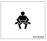
① This lamp lights ON for the first five seconds after starting the truck.
