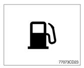
① Fill the fuel immediately when the lamp is turned ON.
