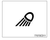
① This lamp lights ON when rear work lamp switch is pressed.
