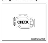
① This lamp light ON during a nonfatal engine system error. The engine can still be run, but the fault should be corrected as soon as possible.
