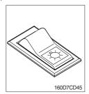
(1) This switch is used to operate the head light by one steps.
